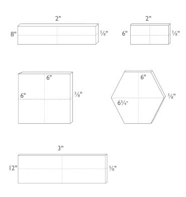
Standard thickness for Pantry Pavers is 3/8"
